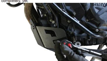
6. Take the four M8x20mm Allen bolts and hand-thread them. Using an M5 Allen key tighten all four bolts.
