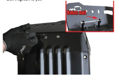
4. Place the bottom metal mounting brackets on the vibration isolation mounts. Short mounting bracket attaches on the back side and the long one in the middle. Using your hand place the M8 nyloc nuts on and turn it by hand a few times then tighten each using a 13mm socket/ratchet combo.
