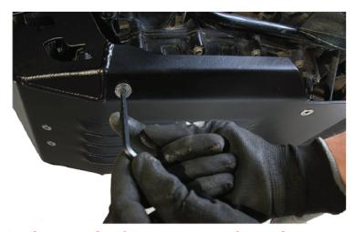
7. Make sure all the bolts are now tightened to the required torque spec by using a torque wrench!
