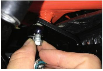
7. Hand-thread the right side factory bolts back into the frame mounting points. Do not tighten it, yet. Don't forget the secure the ball joint on the far end of thesteering damper!
