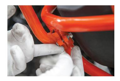
15. Now tie the right and left side crash bars by using the M6x20mm bolts, washers and nuts.
